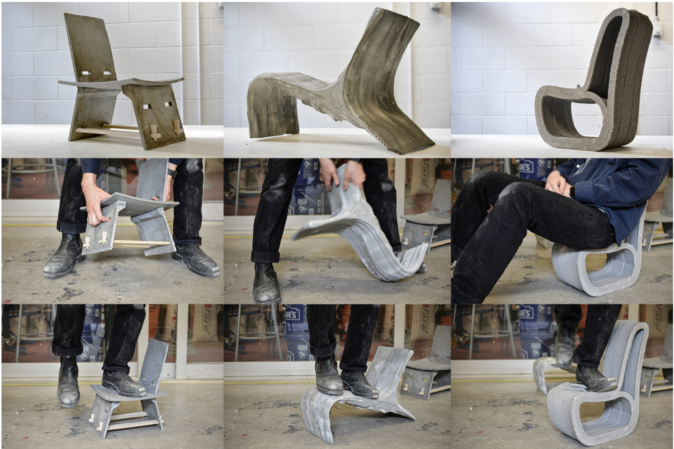
Figure 3. Half-scale prototypes, from left to right: Prototype 1 (cast), 2 (cast + 3D print hybrid) and 3 (3D printed). Image by Sinan Husic
